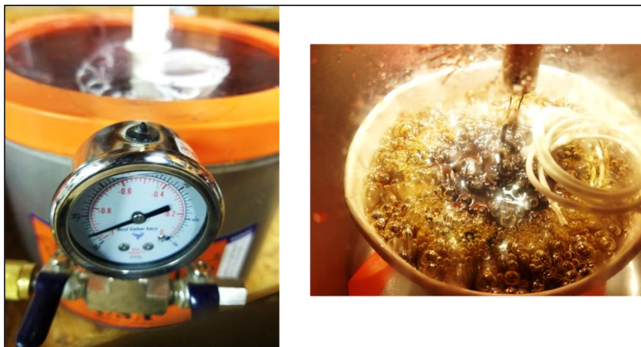
Figure 5.2 Varnish and vacuum impregnation process.
