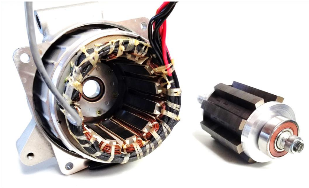
Figure 5.4 SRM stator pressed into housing and rotor fully assembled.
