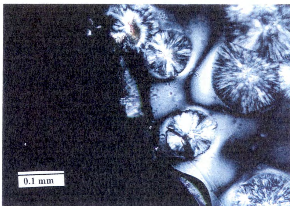
Figure 53: Photograph of spherulites from the FINA specimen (20X).
