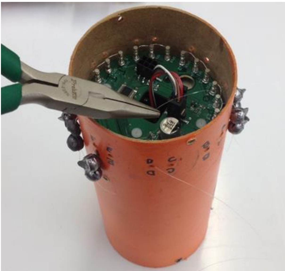
Figure 1. 4: Autonomous Aerial Acoustic Recording System ballast dropper system, showing nichrome wire and ballast weights attached with 6x monofilament line.
