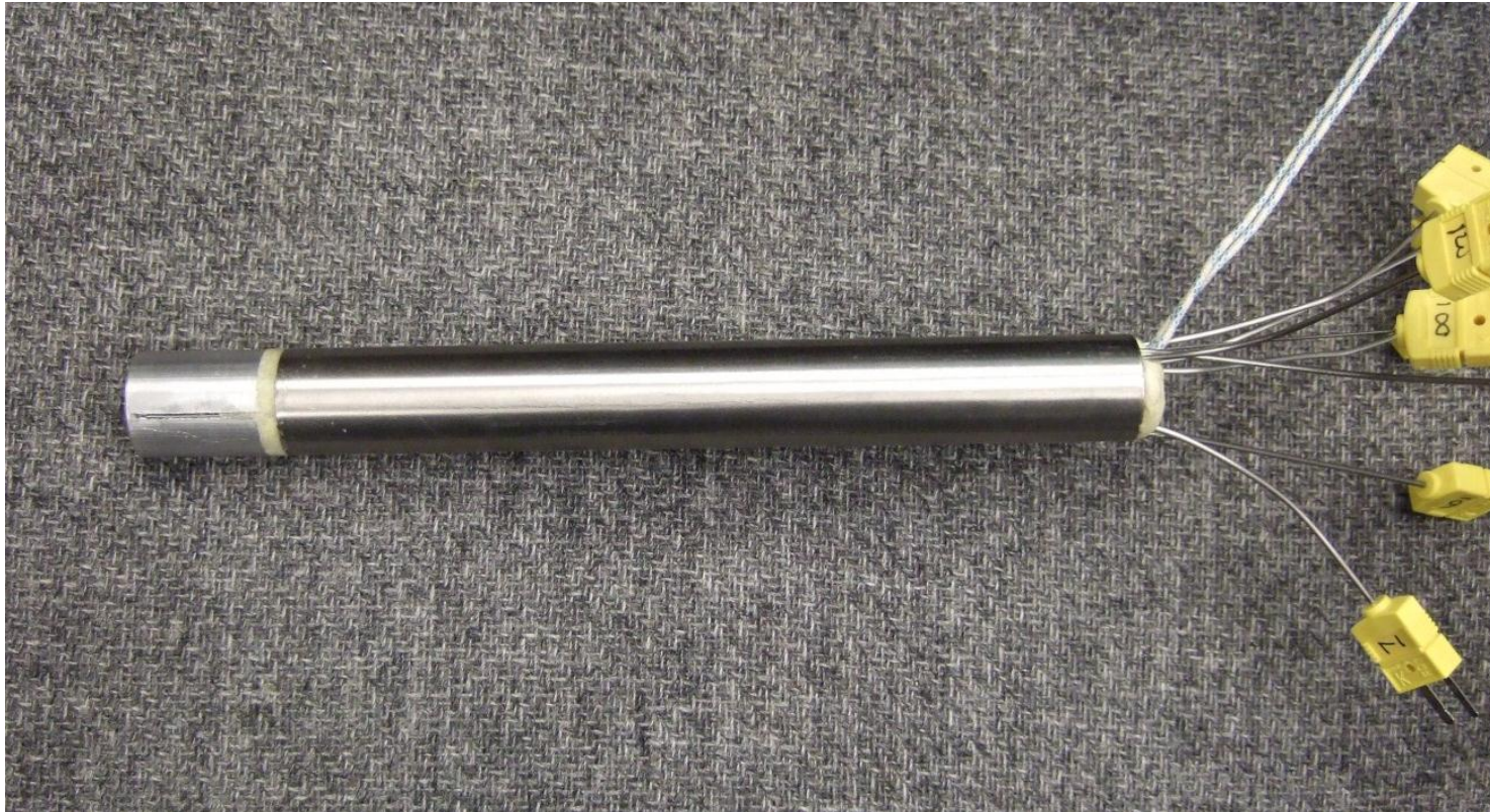
Figure 4: Photograph of the Assembled Simulated Temperature Probe.
