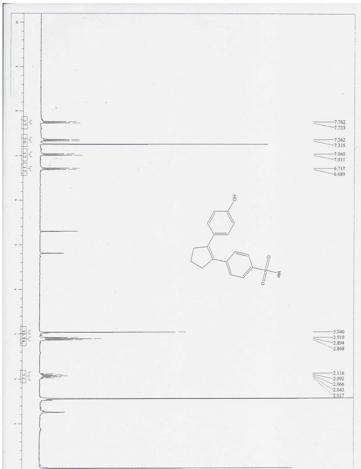
Spectrum 3. Proton NMR of 4-(2-(4-Methanesulfonyl-phenyl)-cyclopent-1-enyl)-phenol, compound 6 , at 300 MHz.
