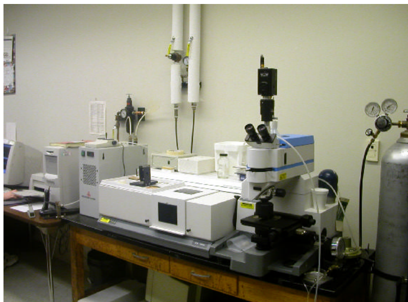
Figure 3.6 Fourier transform infrared spectrometer Bio Rad FTS 6000
