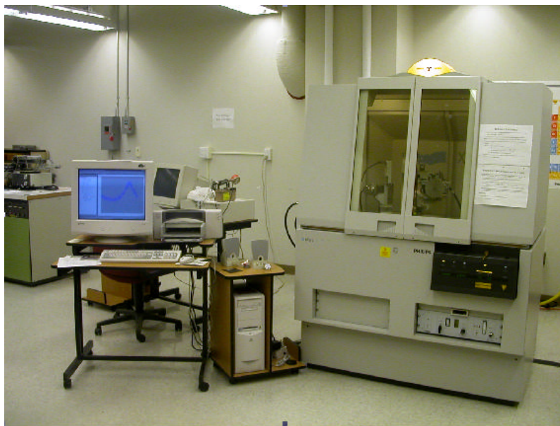
Figure 3.5 Philips x'pert X-ray diffractometer
