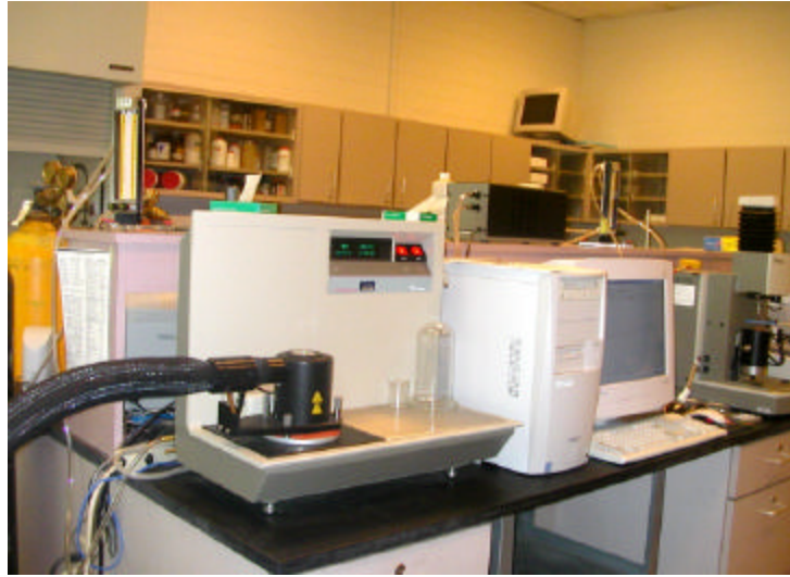
Figure 3.4 Differential Scanning Calorimeter TA instruments 2590
