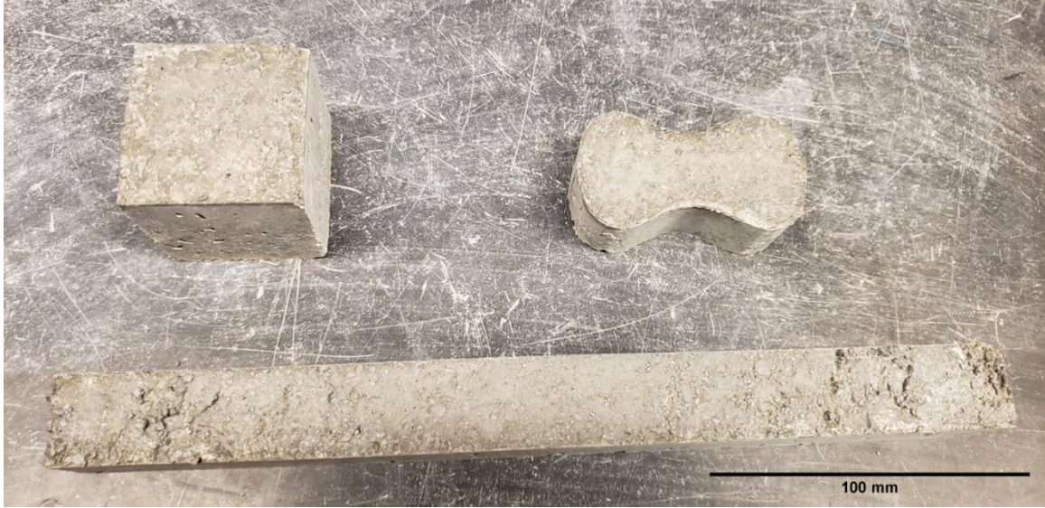
Figure 13: Samples used for mechanical testing. A: compression cube; B: tension briquettes; C: flexural beam.
