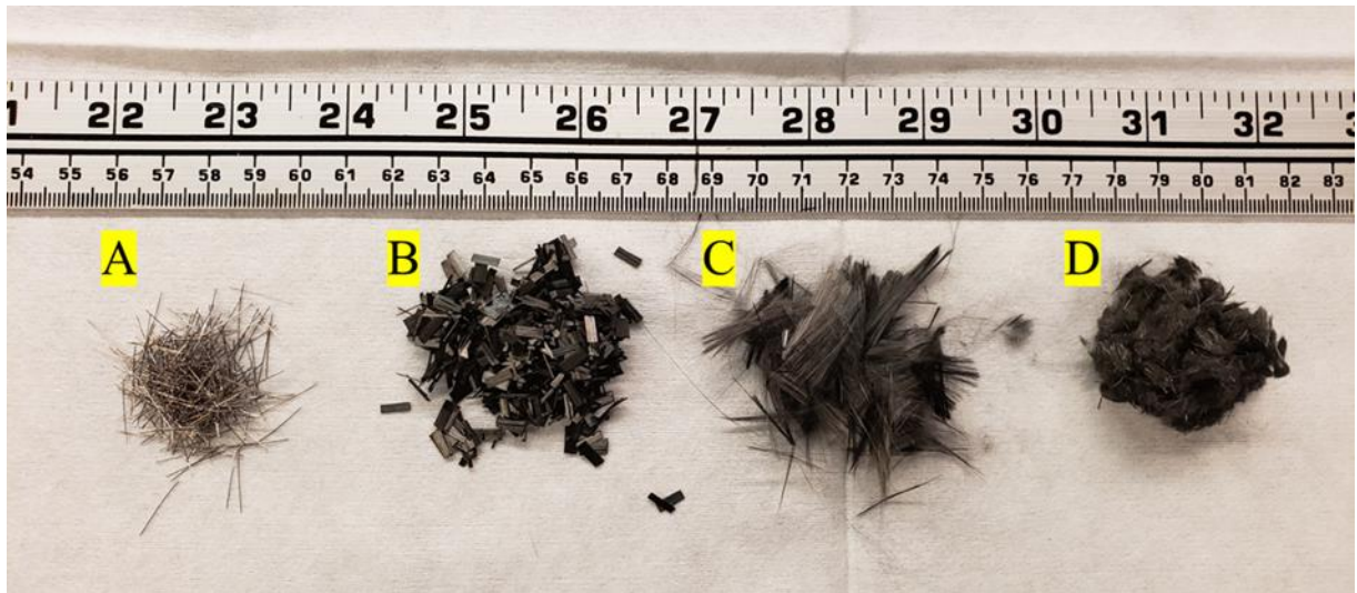
Figure 1: Different fiber types mixed into concrete. A: steel fibers; B: Hexcel carbon fiber; C: Zoltek carbon fiber; D: recycled carbon fiber.
