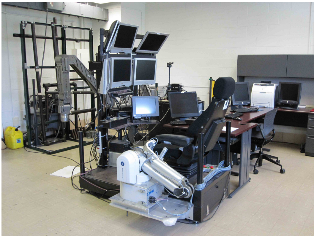
Fig. 48. Remote Console Station.
