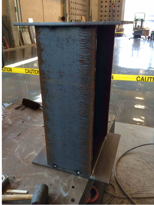
Figure A.3: Unpainted assembled steel support
