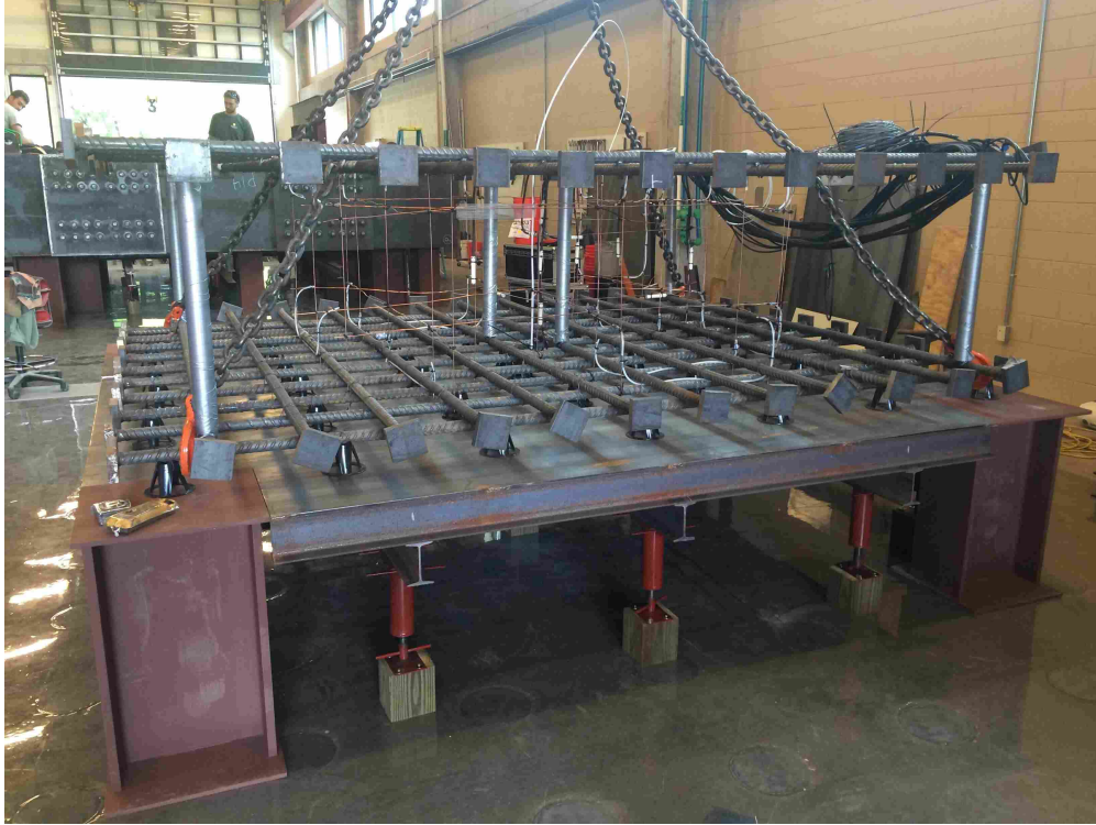
Figure A.5: Completed construction of the bottom formwork with cage in place
