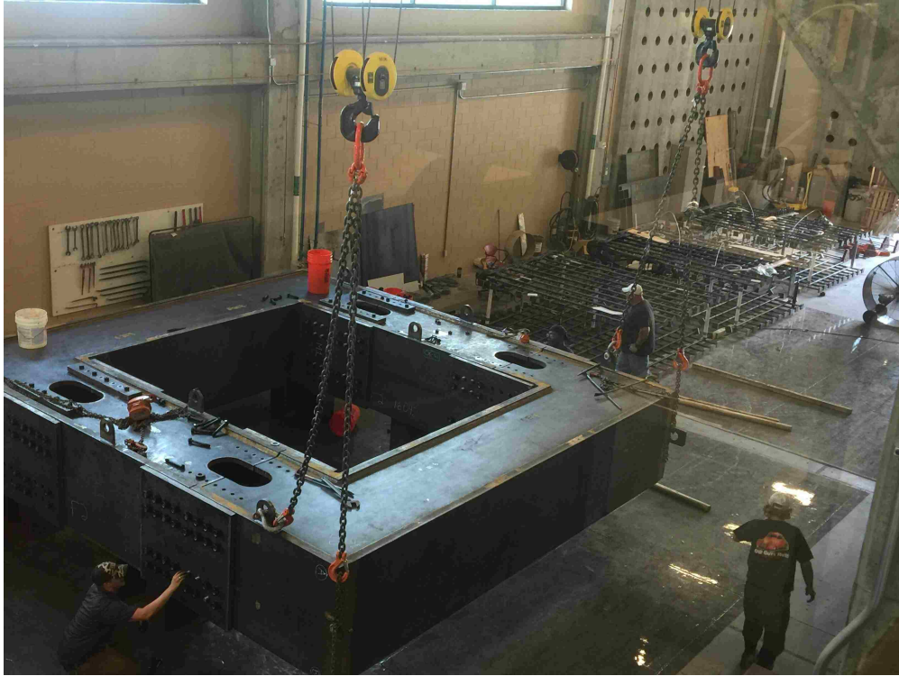
Figure A.8: Assembled steel confinement frame
