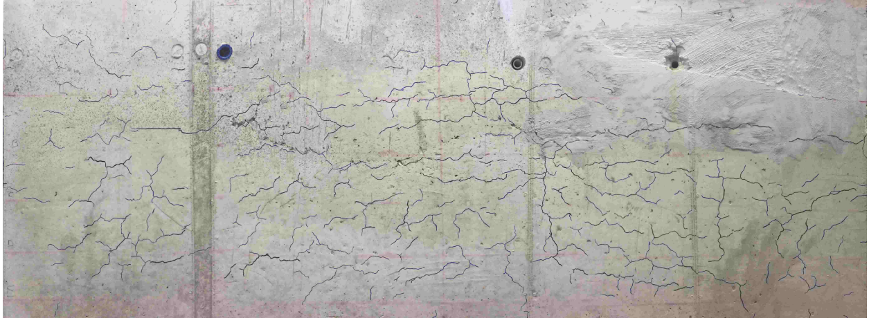
Figure 2.13: Cracking on a side of the UASR specimen Note: Image shown is one side of specimen (3.5 m × 1.0 m)
