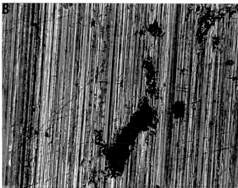
Appendix F.3. Pits observed on the SS metal surfaces. A. SS surface exposed to NR B. SS surface exposed to DR.
