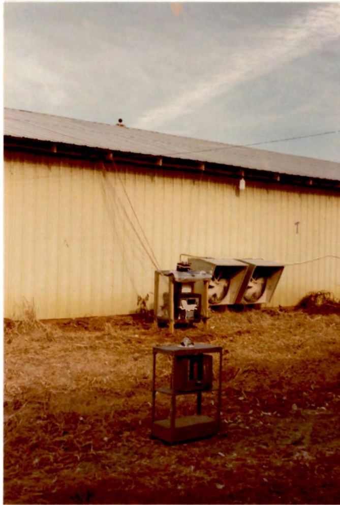
Figure 11. Instruments Used to Measure and Record Temperatures, Solar Radiation, Relative Humidity, and Wet Bulb Temperature. The Pyranometer and Hygrothermograph are in the Foreground. Other Recording Equipment is Located in the Shelter Near the Fans. Note the Black Globe Sensor on Top of the Building.
