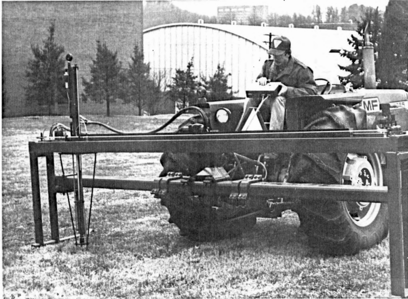
Figure 1. Rear view of soil cone penetrometer mounted on a 46 PT0 Kw agricultural tractor.
