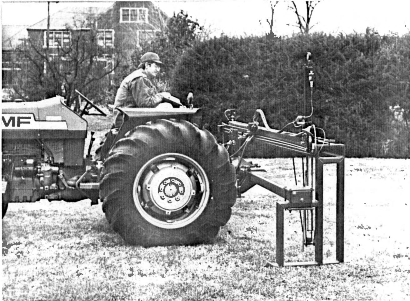
Figure 2. Side view of soil cone penetrometer ready for use in the field.
