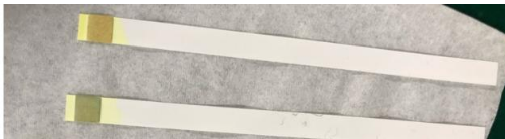
Figure 2.4. Photograph showing peroxide test strips after being dipped into the solution prior to irradiation (top) and after 10 minutes (bottom) during the photomodification of 2.1 under ambient atmosphere.
