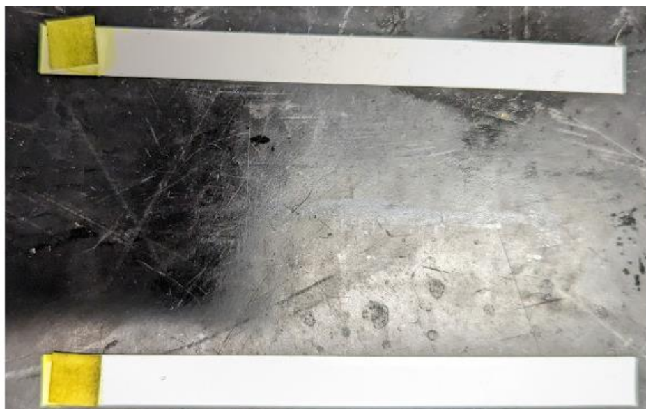
Figure 2.5. Photograph showing peroxide test strips after being dipped into the solution prior to irradiation (top) and after 10 minutes (bottom) during the photomodification of 2.1 under N 2 .
