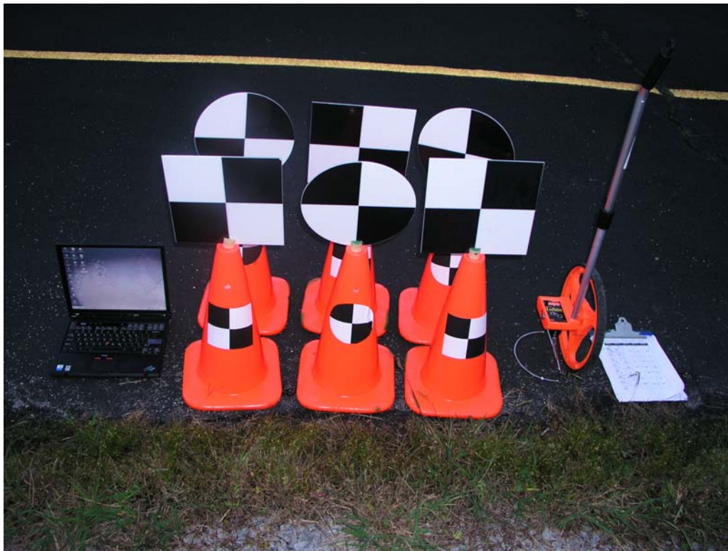
Figure 3. Equipment Used For Photogrammetry Experiment
