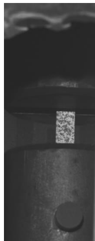
Figure 3.2 A speckle image of the gauge section of creep specimen
