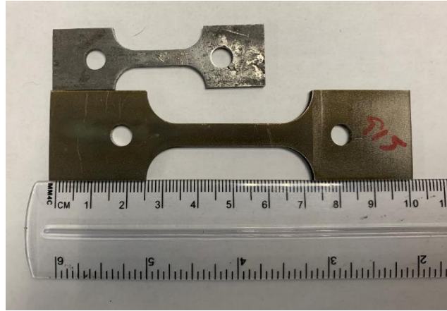
Figure 8.3 Photo of traditional manufactured creep specimen (top) and mBAAMed creep specimen (bottom)
