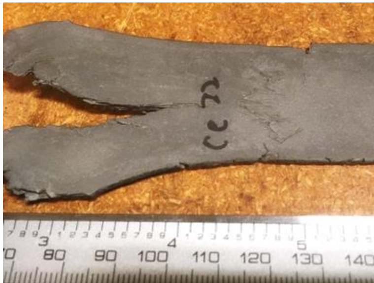
Figure 8.1 As-rolled FeCrAl sheet with visible cracks
