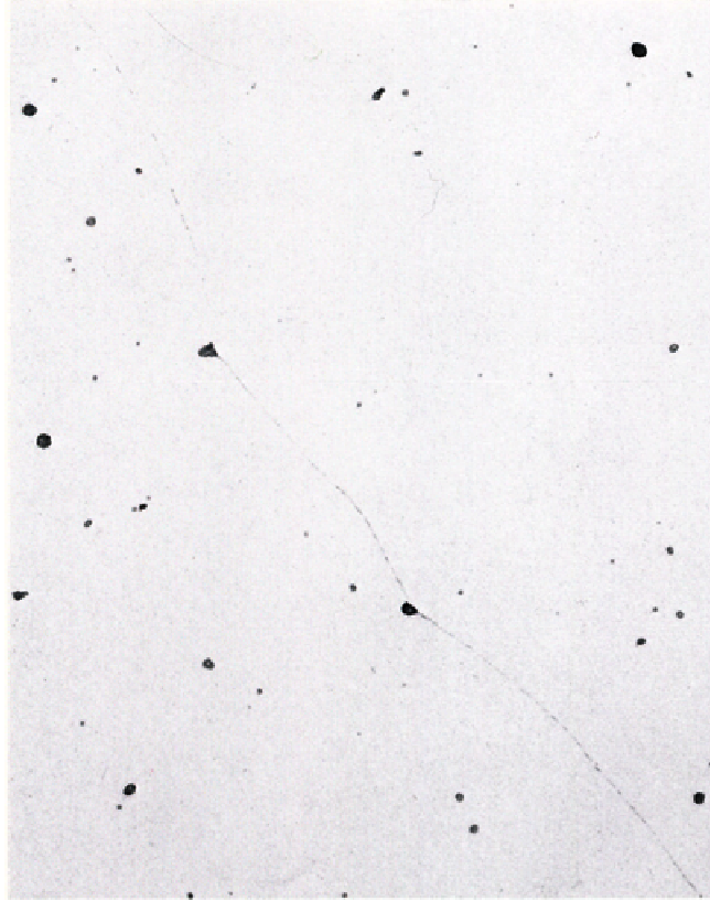
Figure 11: Solution treated 1 hour at 2150 °F (1175 °C), water quenched (correct heat treatment) shown at 200 x magnification showing austenite with dispersed inclusions. Oxalic acid etch.
