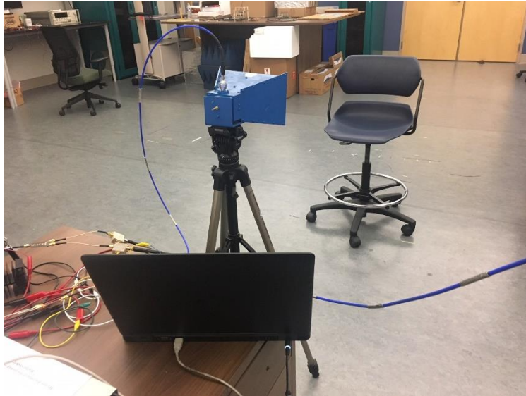
Figure 2.28 Mono-static SFCW radar system for human vital sign detection.
