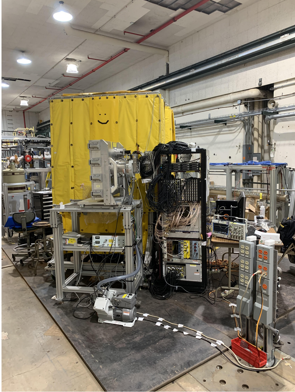
Figure 4.2: Picture of MTAS at Argonne National Laboratory. MTAS is located behind the yellow lead shielding blankets. In the front of the picture on aluminum framing is the Moving Tape Collector (MTC). To the right of the MTC are the switchboard and Pixie digitization modules, along with other NIM modules. Below the MTC a roughing pump can be seen, which along with the turbo pump mounted at the MTC, ensure that the MTAS center tube is operating in vacuum.
