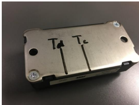
Fig. 5-54. Phase-leg module and the thermocouple locations
