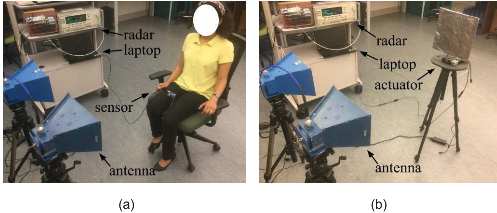
Figure 2.5 Experiment setup with (a) human subject, (b) linear actuator.
