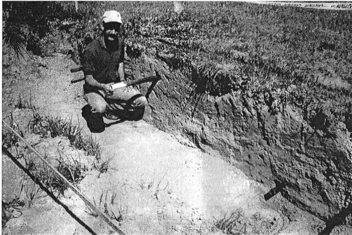
Figure 3.19. Metal rods inserted into the soil profile for calibrating the GPR data and identifying soil features.
