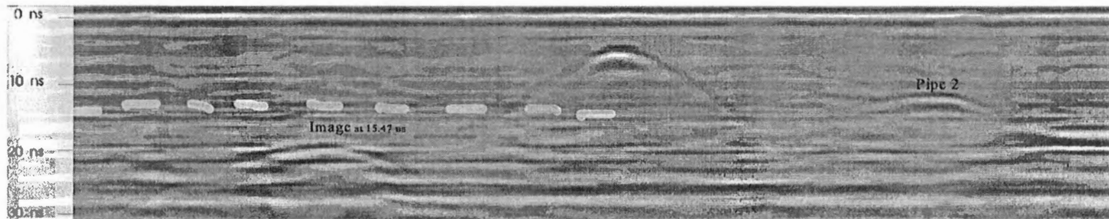
Figure 4.3. Radar reflections at approximately the BC\Cr interface are shown in the image taken with a 900-MHz antenna in test one. The reflection is highlighted with a dashed line on the left side of the image. The location of this 7-m scan, labeled scan 1, is shown in Figure 3.18.
