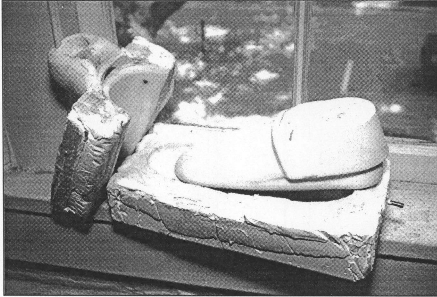
Figure 10. The mold used to make the rubber inserts
