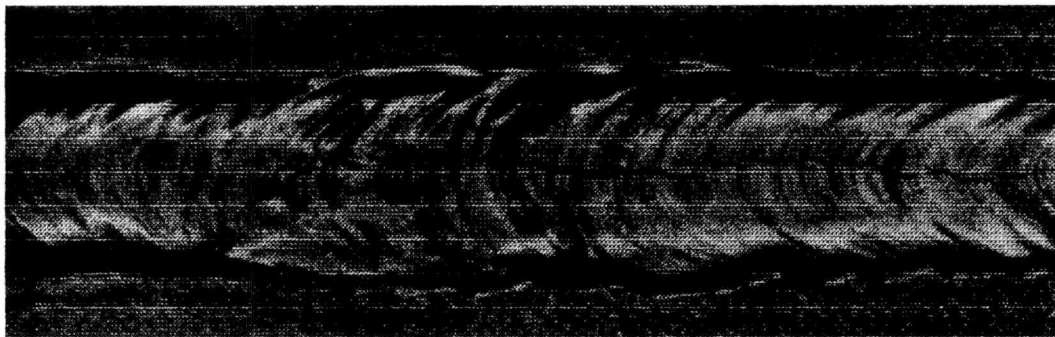
Figure 4. An example of solidification cracking in arc welded aluminum. (Source) J. Knight, Welding Kaiser Aluminum , Kaiser Aluminum & Chemical Sales, Inc, CA, 1967.
