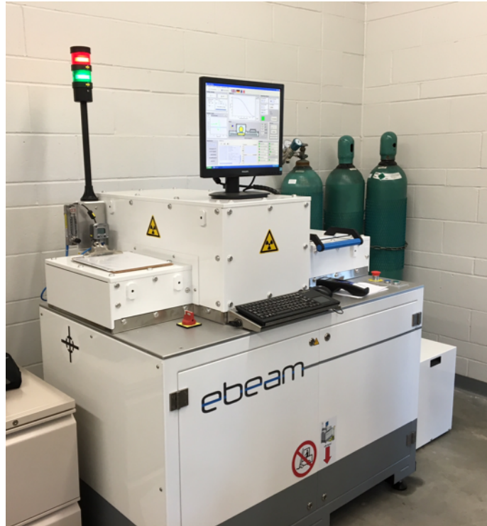
Figure 5.2 EBEAM facility by the Comet Group for laboratory scale e-beam applications.
