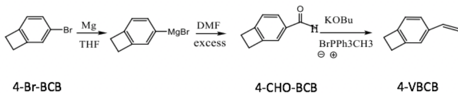
Scheme 3.1 Two-step synthesis of 4-VBCB monomer from 4-Br-BCB precursor including Grignard reaction and Wittig reaction
