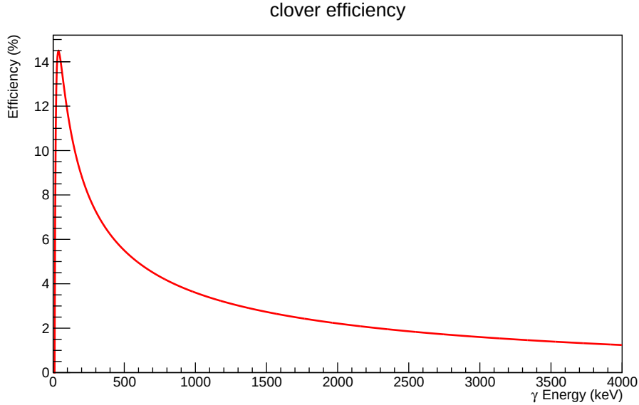
Figure 4.5: The detection efficiency curve for \gamma -ray detection using the 2\pi DEGAi hemisphere consisting of 11 clover detectors. More details are in the text.
