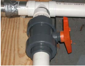
Figure 2: Flow velocity control device, PVC 3 inch ball valve.
