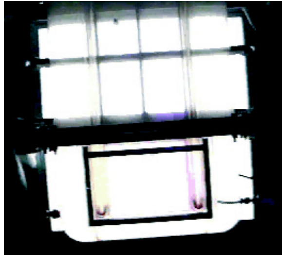
Figure 9.2 – Flow visualization study in the modified WTHL test section with dye injected along the inside surface of the flow vane. The flow rate is half of the nominal flow rate (5.5 l/s per inlet leg). To see video footage of this experiment, click on the image to activate the animation.
