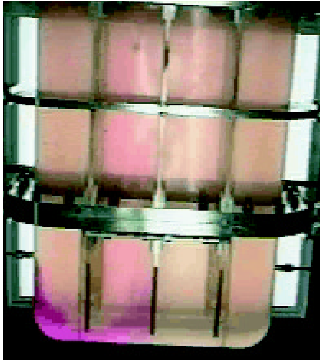
Figure 6.7 – Flow visualization in the WTHL test section at half-nominal flow using dye injection. To see a video recording of this experiment, click on the image to activate the animation.
