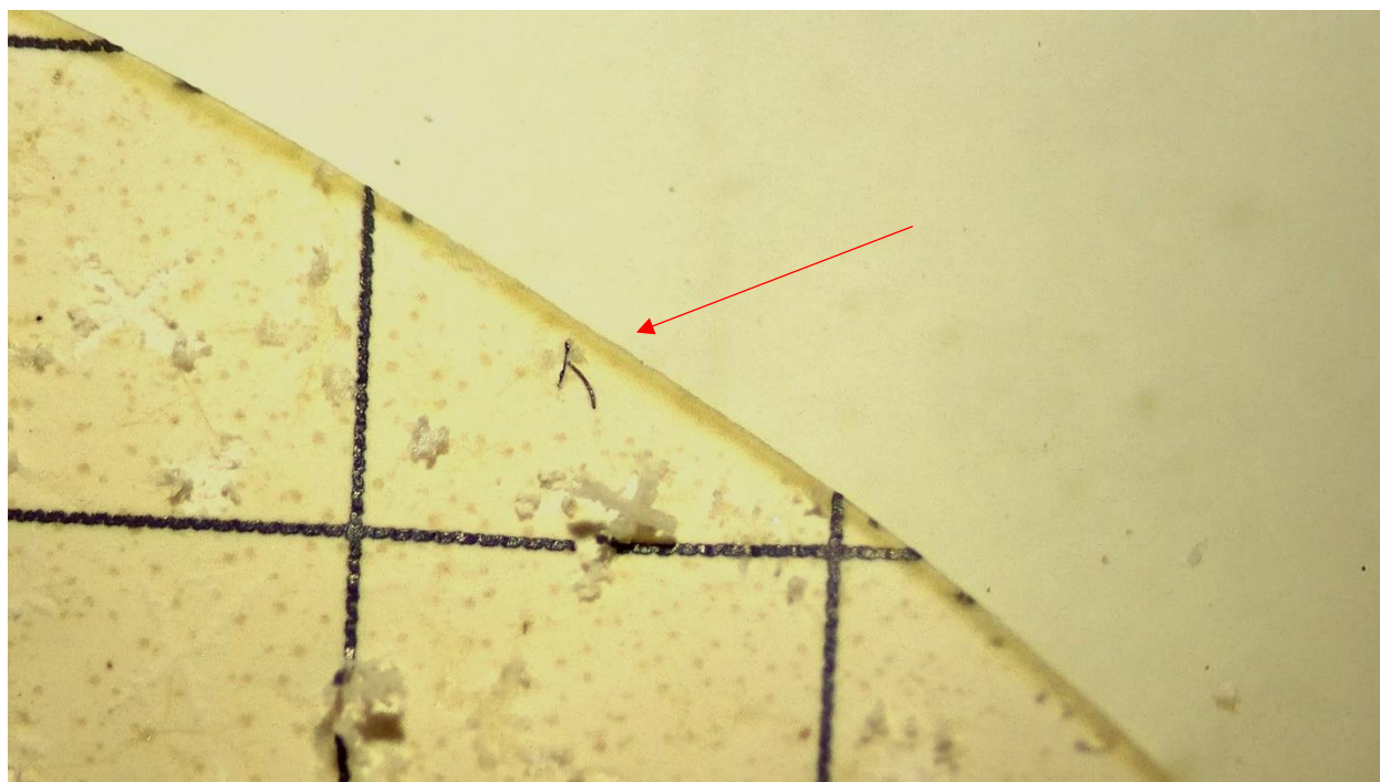
Figure 15 Filter grid line that has peeled away from chemical digestion
