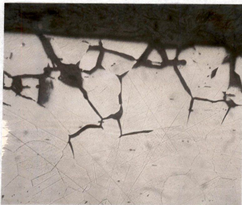
Figure 17. Photomicrograph of Heat LWH7T. Longitudinal Sample - 200X - Oxalic Etch.
