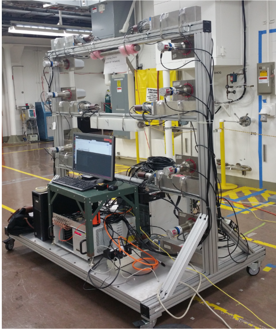
Figure 3.3: DANG: Detector Array for Neutron and Gamma detection.
