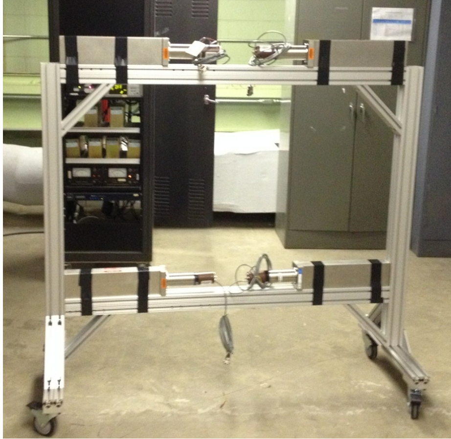
Figure 3.2: 2 x 2 array of NaI bricks. Detectors on a row are 40 inches apart, first row is 21.5 inches off the ground, second row is 60 inches.
