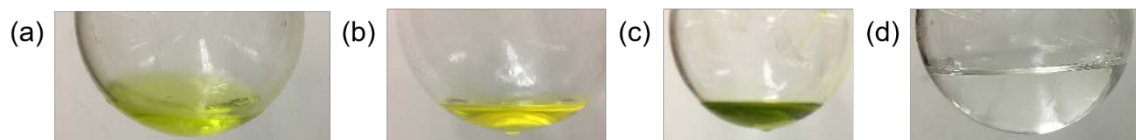
Figure 4-1. Reaction solutions on the synthesis of PMMA macromonomer: (a) activation of PVBA by sec -BuLi upon mixing; (b) the completion of the activation of PVBA by sec -BuLi; (c) formation of a complex between LiCl and nitrogen anion; (d) Solutions of living PMMA.
