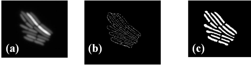
Edge detection based on 'log' filter of fluorescent images Laplacian of Gaussian
