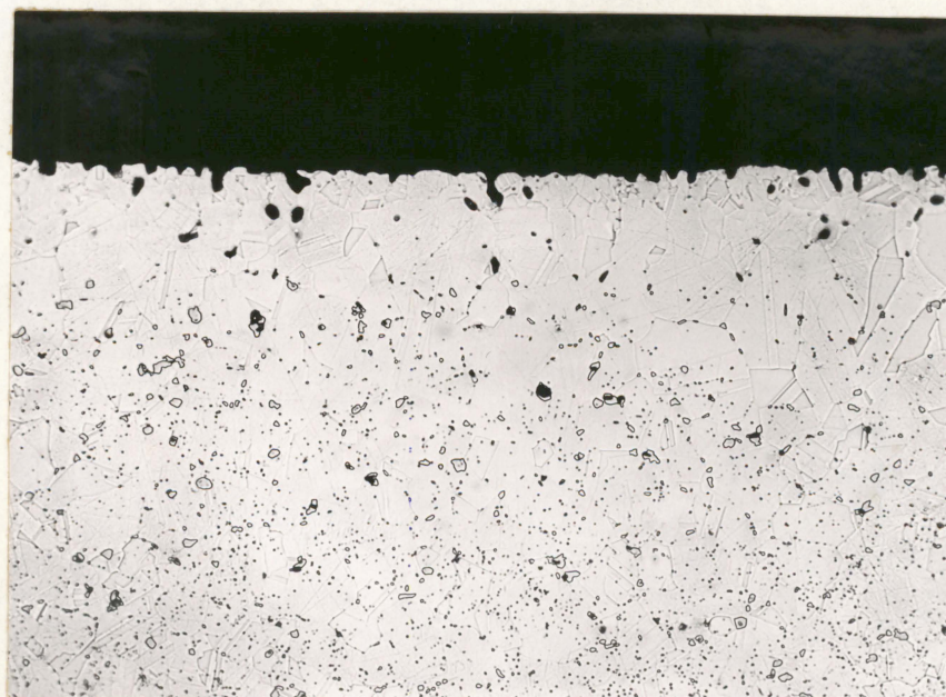
Hot-Leg Section ( 857^{\circ}\text{C} ) Corrosion Rate: 0.92 \text{ mg/cm}^2
