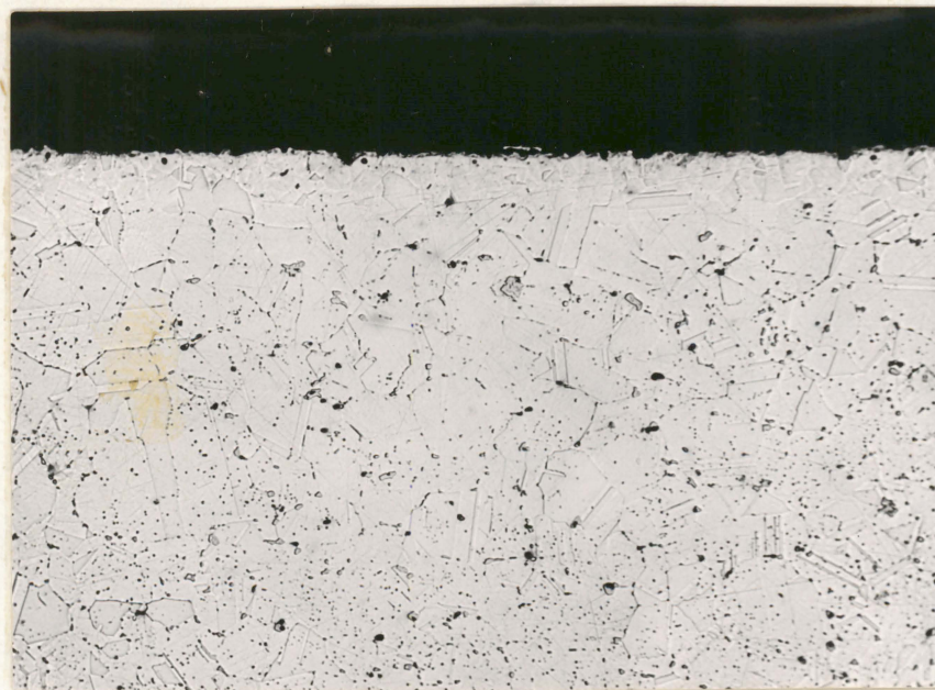
Cold-Leg Section ( 684^{\circ}\text{C} ) Corrosion Rate: 0.14 \text{ mg/cm}^2
