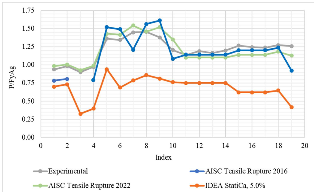
Figure 4.5: Round HSS results: strength ratio vs. index
