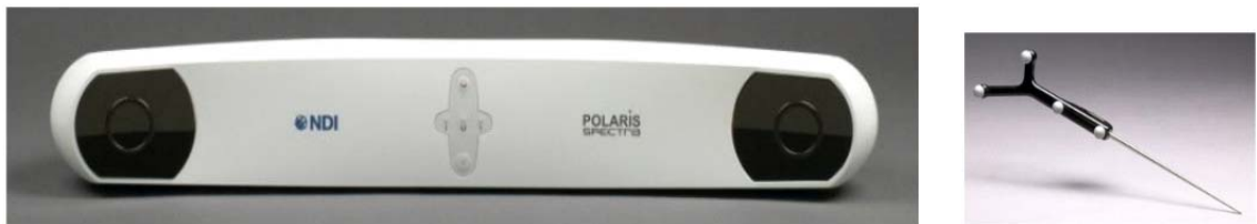
Figure 1-1: Polaris Spectra optical tracking system from Northern Digital Inc. (a) optical receiver, (b) passive optical probe with four reflective markers [5].
