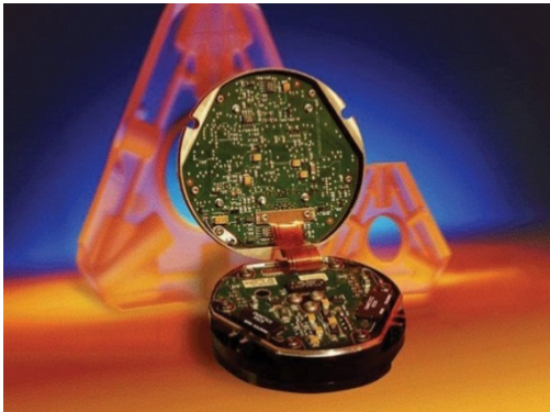
Figure 3-8 - GG1320 ring laser gyros for military aircraft inertial system [74]
