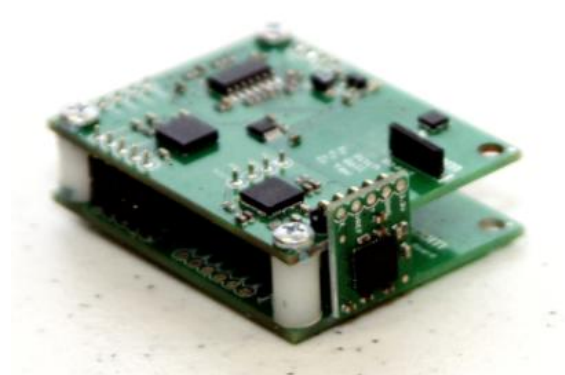
Figure 3-9 - MEMS based strapdown IMU by Sparkfun Electronic
