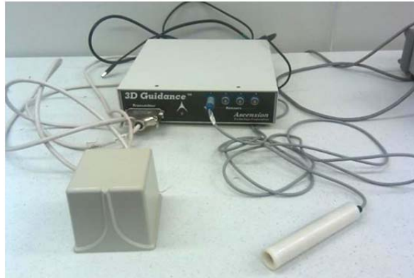
Figure 1-4 - Magnetic tracking system from Acension Technology [12]
