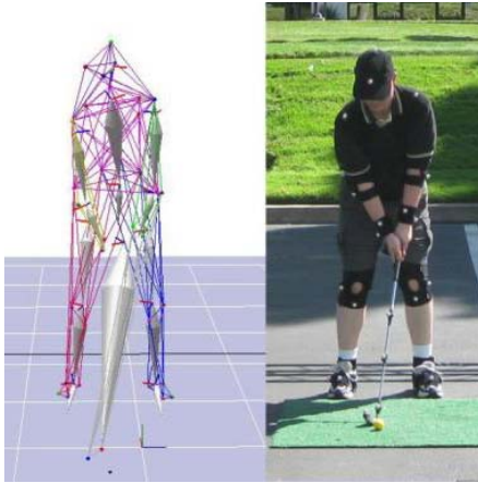
Figure 1-2 - Passive marker optical tracking system from Motion Analysis Corporation showing the capability of motion capture during ambient sunlight [6]
