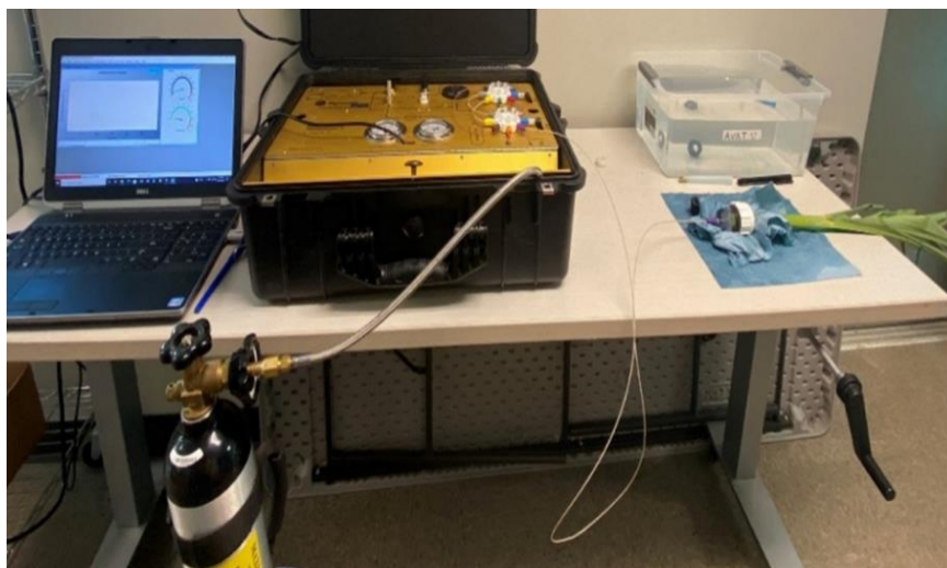
Figure 2. Measurement of shoot hydraulic conductance ( K_{\text{shoot}} ) using a hydraulic conductance flow meter (HCFM)
