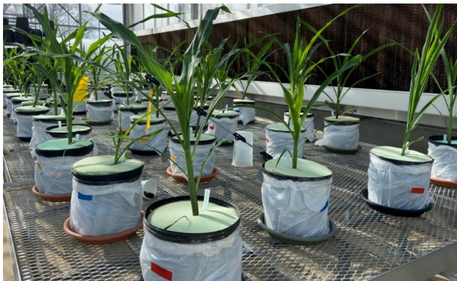
Figure 1. A greenhouse setup where each pot's mouth was sealed with 7.6 cm thick foam and placed into doubled-bagged 15 L plastic bags to allow water loss only through transpiration during the soil dry-down study
