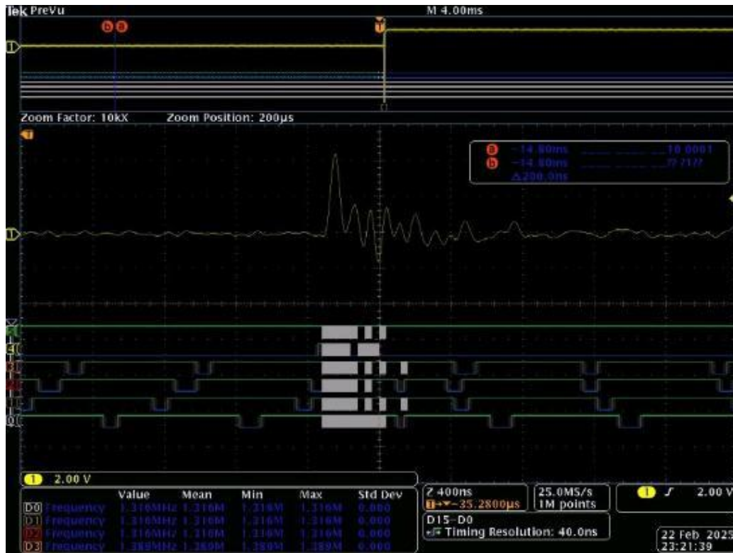
Figure 7.10. Voltage sensor feedback signal D0-D3 all interrupted.
