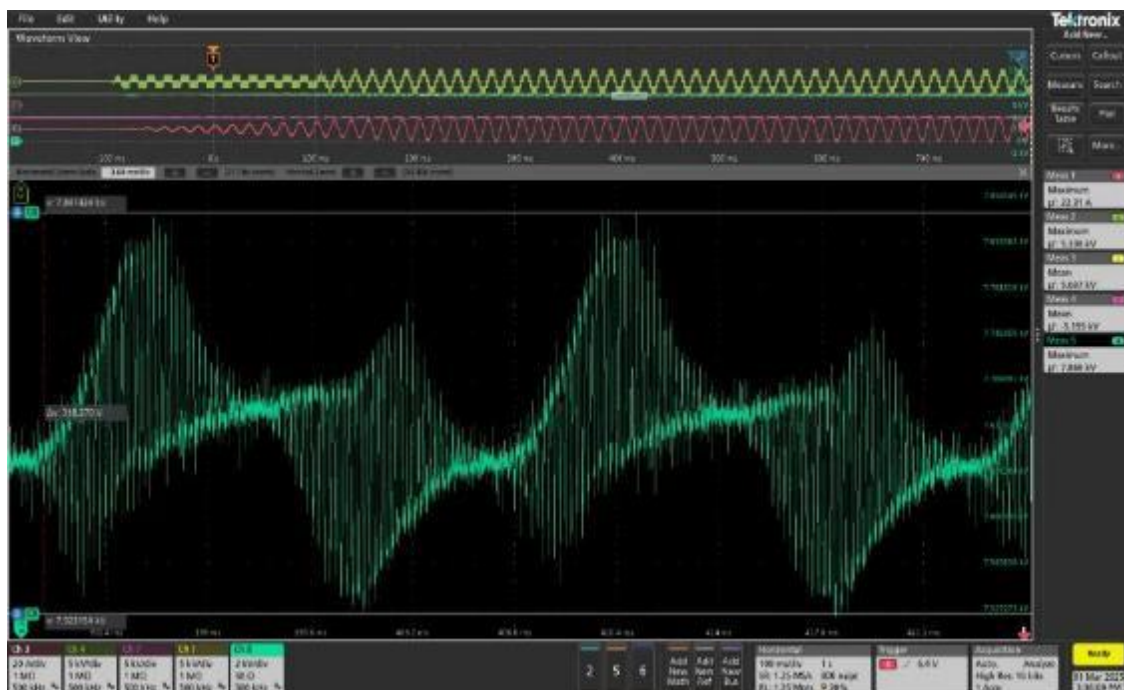
Figure 7.12. 3 rd stage flying capacitor voltage ripple at 10 kV dc link voltage.
