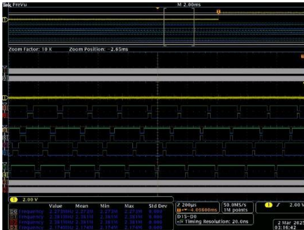
Figure 7.14. Gate PWM signals are clean at 22 kV after measures implemented.
