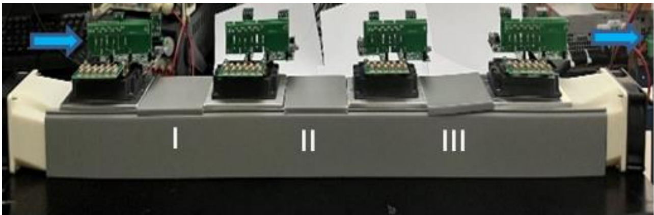
Figure 5.18. Air flow velocity measurement locations.
