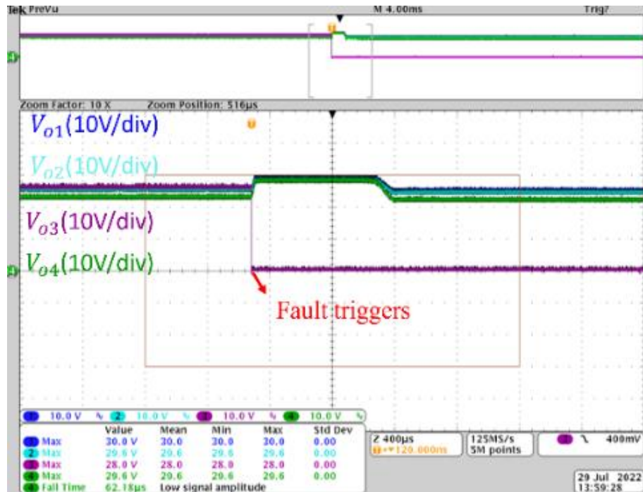
Figure 3.14. Short circuit is cleared by secondary protection.
