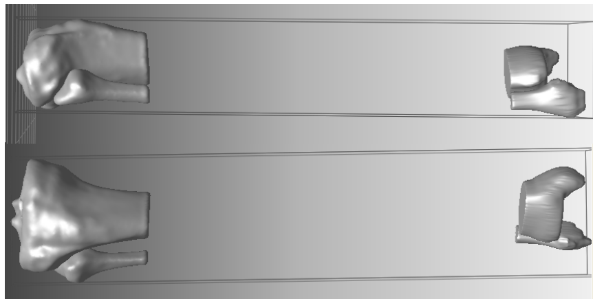
Figure 39: Lateral (top) and frontal (bottom) views of the CAD model of the femur developed from CT scans of a single subject (Subject 3) as viewed in RapidForm2006 (Inus Technologies, Inc., Seoul, Korea) with model bounding boxes. The position of points such as the knee ligament, quadriceps and hamstring and medial and lateral patellofemoral ligaments attachments and the center of the femoral head are found by using anatomical landmarks, if visible, or using guides from literature. The center of mass is also calculated using the size of the segment and formulas from literature. The shaft of the femur is not continuous as CT scans were only performed on the areas visible in the image. Any points needed in the area of the model which is not available are estimated.
