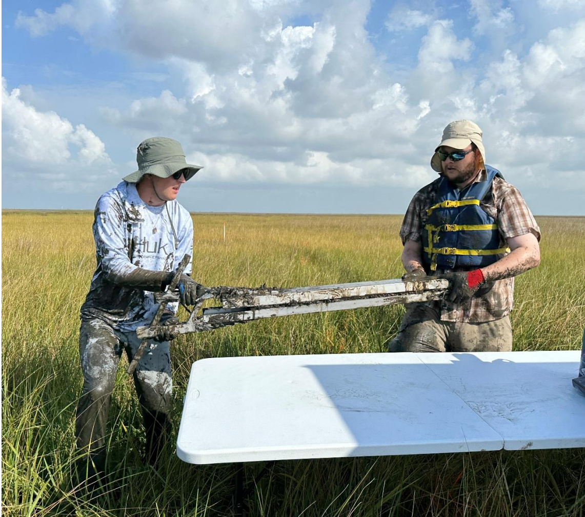
Figure 2.2. A photograph immediately following core extraction using the Wardenaar Peat Profile Sampler.
