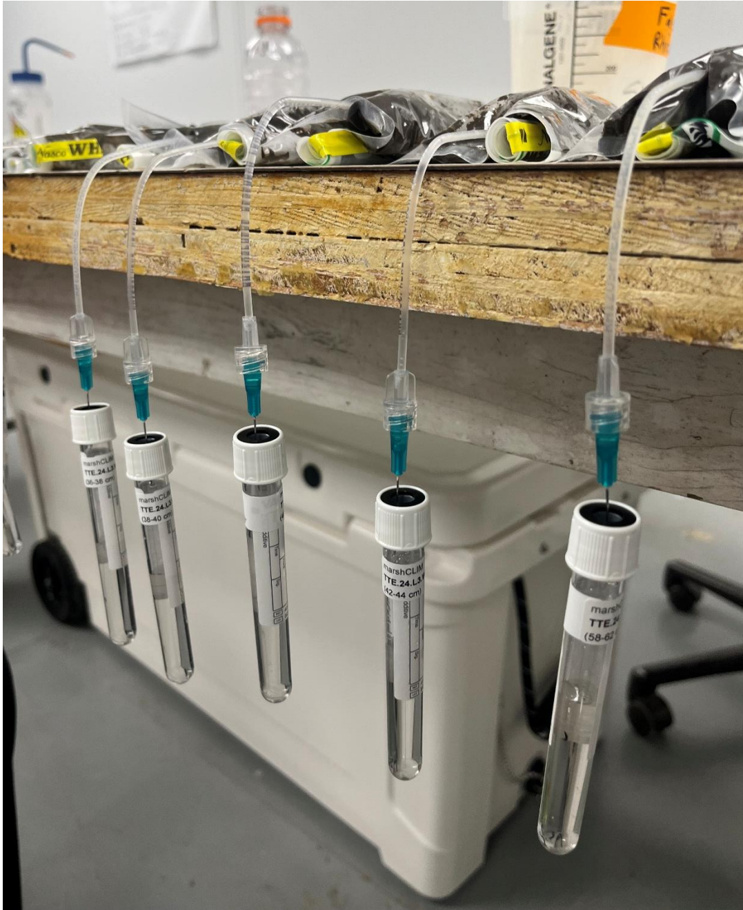
Figure 2.4. Porewater extraction from soil in a Whirl-Pak bag with an attached Rhizon, needle, and Vacuette vial after samples were transported from the field to the laboratory.
