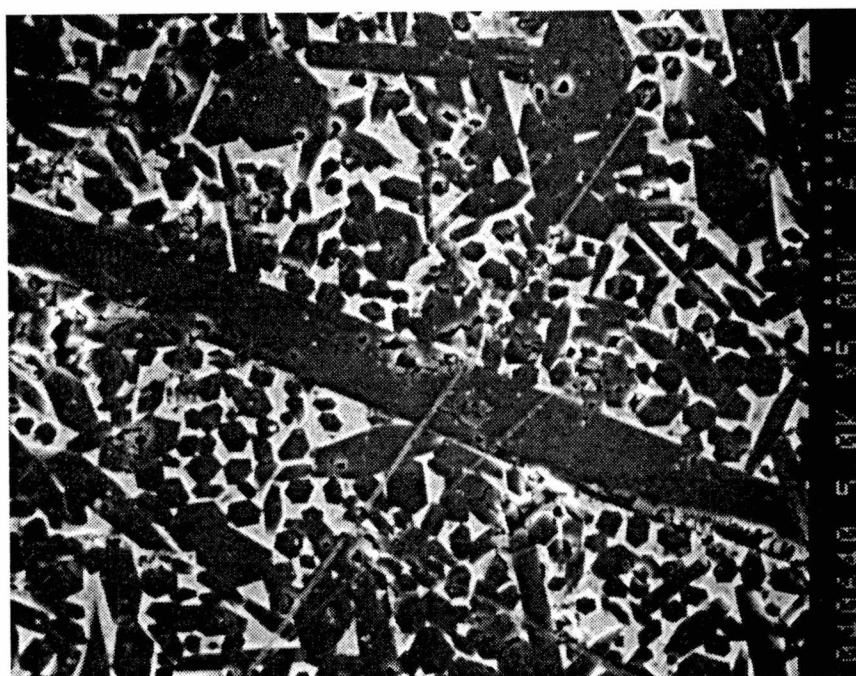
Fig. 3.21. Etched surface of sample TRSN-45-13 showing microstructure variation from the as-sintered surface into the specimen interior. (a) Near as-sintered surface, (b) \sim 1 mm from as-sintered surface, (c) \sim 2 mm from as-sintered surface and (d) \gg 2 mm from as-sintered surface in the bulk of the material.
