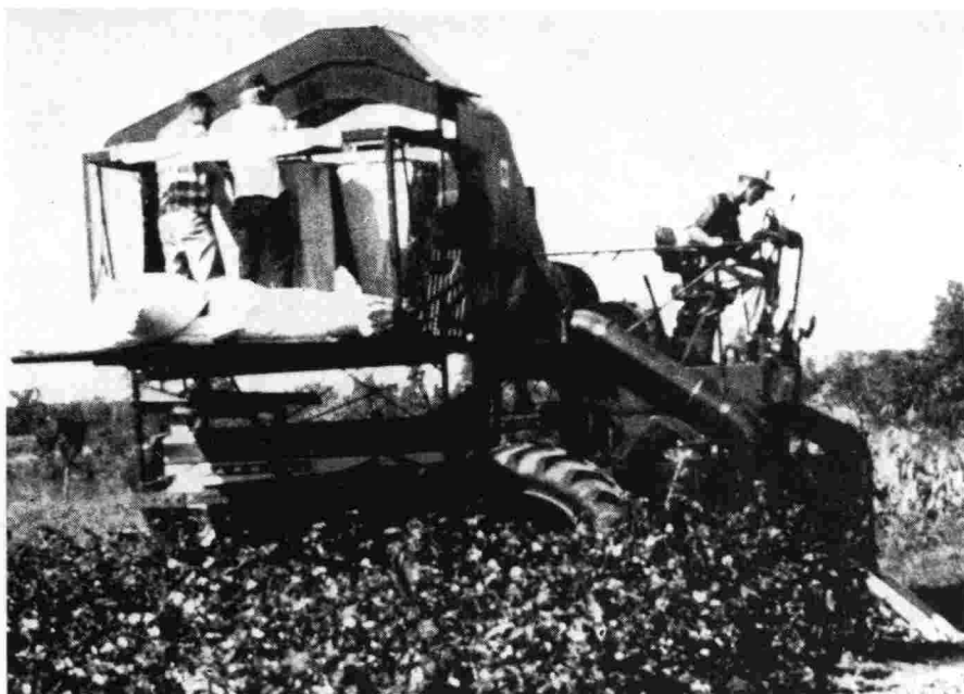
“Harvesting cotton plots with one-row spindle picker equipped with a special sacking attachment for collecting samples,” 1968 Annual Report, page 16.
