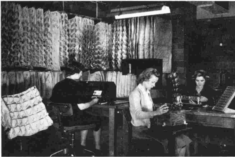
"Fiber research laboratory, showing operators measuring fiber length with the fibergraph (left), fiber fitness with the arealometer (center), and fiber strength with the Pressley instrument (right). Such tests also are made available to the industry through the Fiber Testing Service, thus combining research with its application," 1941 Annual Report, front cover.
