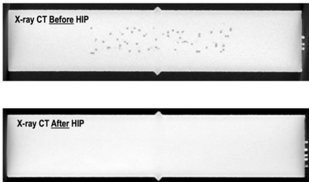
Figure 3-5: XCT data highlighting closure of pores after HIP/SA in two representative slices.
