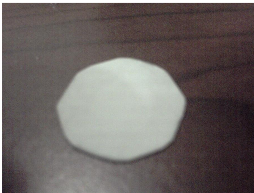
Figure 67. Small ceramic piece used to electrically insulate the sample from the heater
