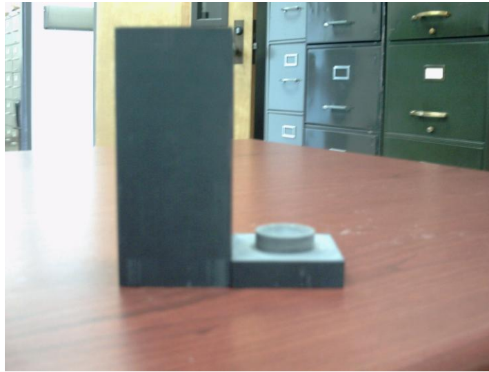
Figure 2. Top and bottom ceramic block for insulating the samples
