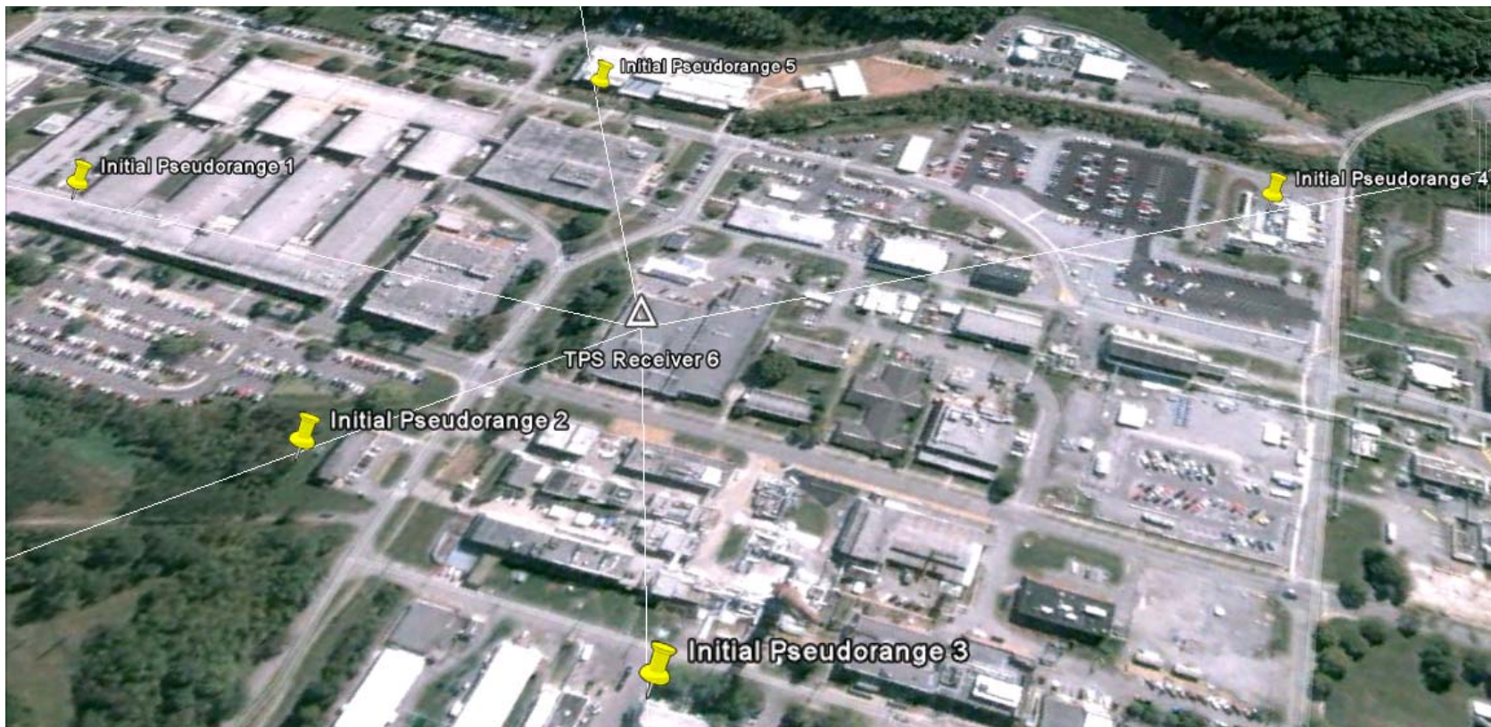
Figure 5 – Approximate physical locations of initial pseudoranges relative to TPS receiver site 6
