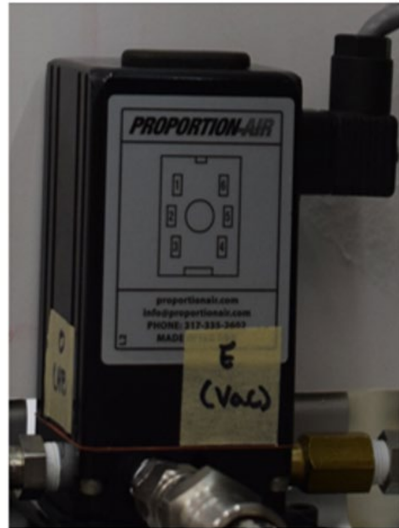
Figure 4.13: (Left) 0-10 VDC potentiometer and (Right) QB1X pressure controller.
