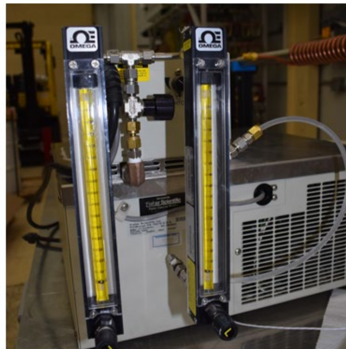
Figure 4.20: (Left) ISOTEMP 1006D circulator with control box, (Right) ISOTEMP 1006D with Omega rotameters.
