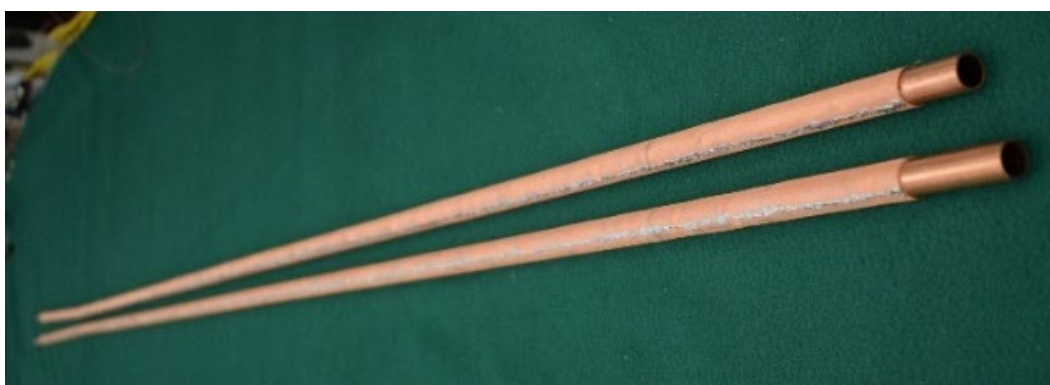
Figure 4.2: Fabricated copper wicks.
