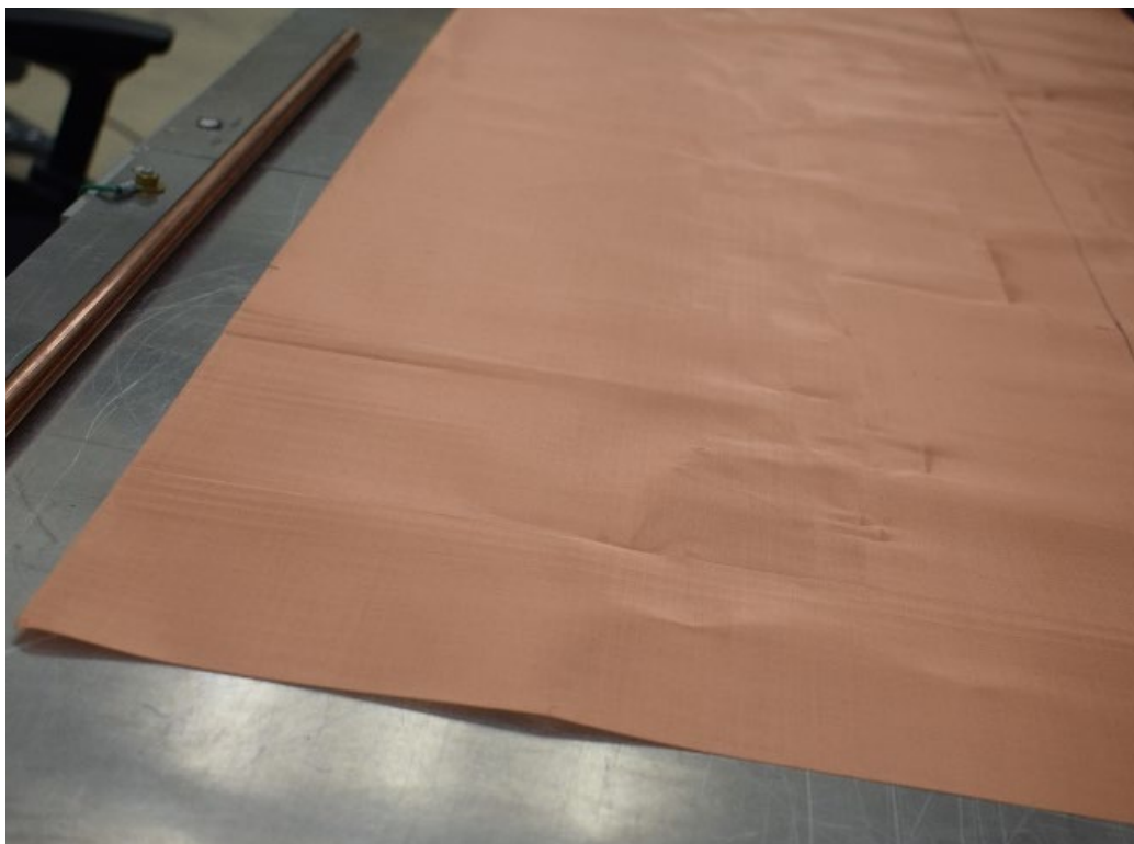
Figure 4.1: 100 X 100 copper mesh material.
