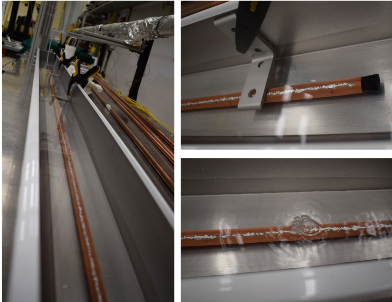
Figure 4.4: Bubble point test in water.
