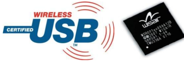
Figure 2-15: Wireless USB is now a certified technology which utilizes UWB MB-OFDM for high data rate digital communication. Commercial chipsets and products are available, including the CMOS chipset from Wisair which is commercially available in a range of products [92].
