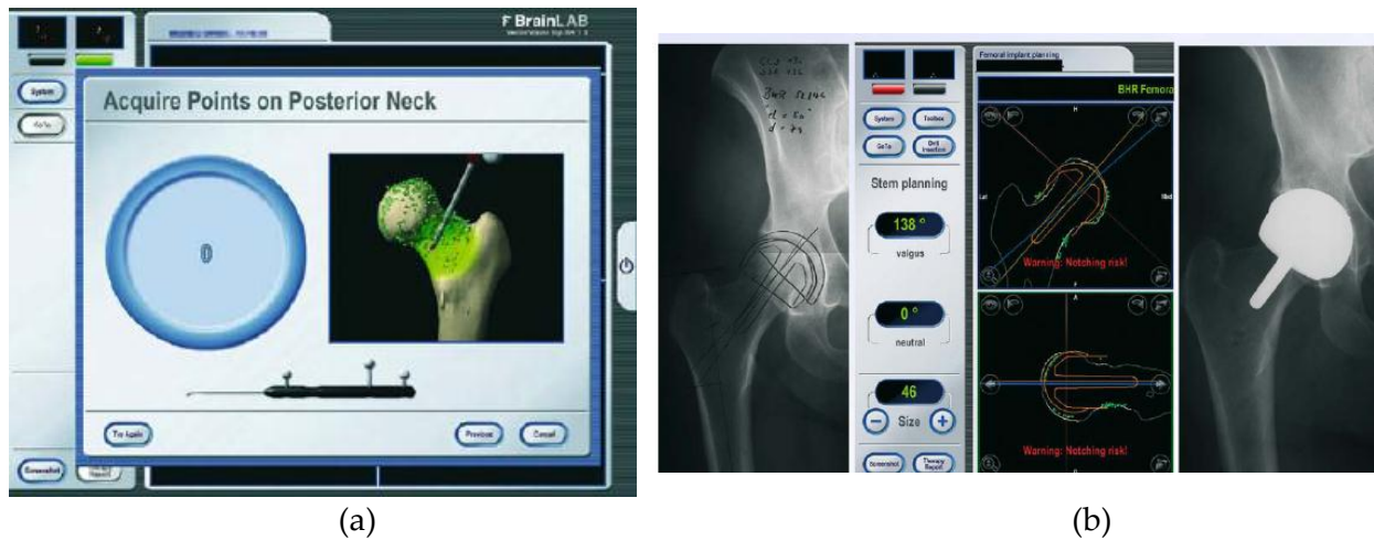
Figure 3-15: (a) BrainLAB VectorVision® Navigation System software interface for picking points on the neck and head of the femur [136], (b) Smith and Nephew Birmingham Hip Resurfacing system software interface post-operative validation [137].
