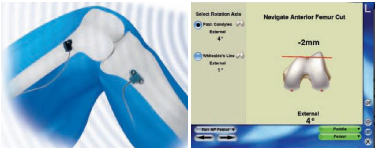
Figure 3-11: Medtronic knee navigation system highlighting AXIEM™ electromagnetic tracking sensors and software interface for selecting where to make the anterior femoral cut [106].
