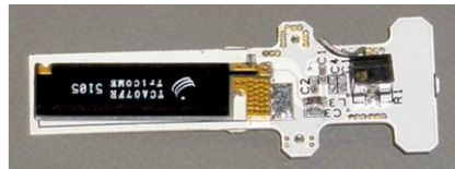
Figure 2-12: Transmitter for in vivo wireless telemetry which uses a MAX1472 ASK transmitter operating at 433 MHz connected to a chip antenna to transmit digital information.
