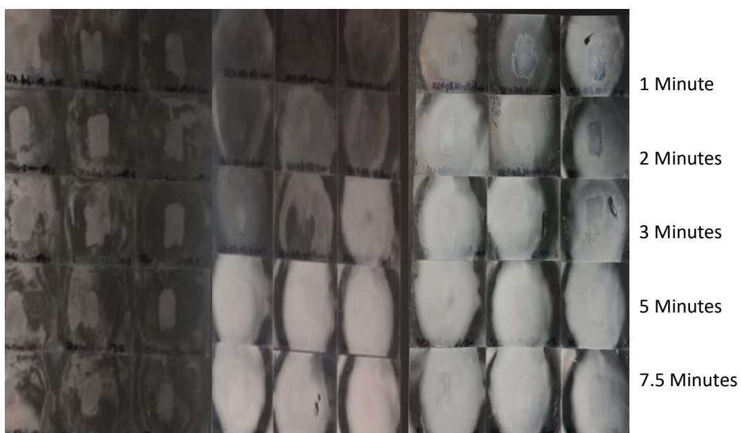
Figure 2-5: Photos of slides after fuming at a surface temperature of 10 °C at ambient (left), 50% (middle) and 80% (right) relative humidity over time.
