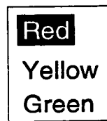
Figure 2.2: The feedback object in this menu uses constraints with pointer variables to 1) position itself over the selected object, and 2) resize itself to match the dimension of the selected object. By changing the value of the variable obj-over , the feedback object can appear over any object in the menu. obj-over currently points to the red menu item.
