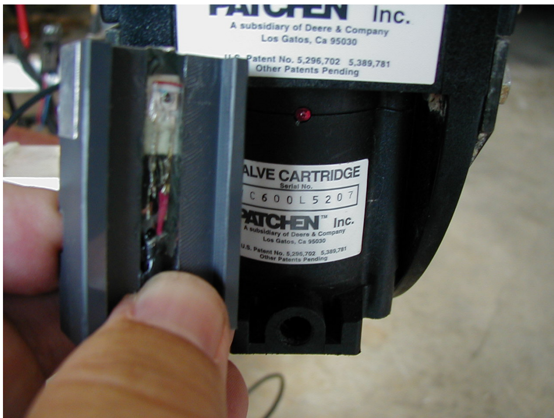
Figure 4. A photograph of a WeedSeeker valve cartridge and the phototransistor potted in a milled plastic block used to monitor the valve status.
