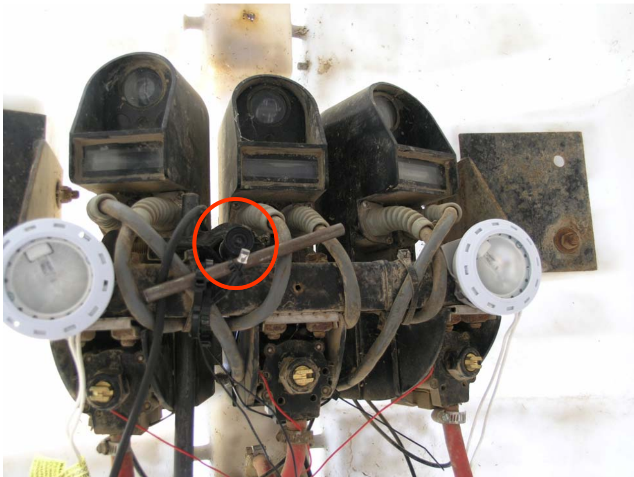
Figure 5. Photograph illustrating the underside of a three WeedSeeker cluster mounted in a spray hood, video camera, LED, and supplemental lighting used during testing in Stoneville, MS (July 2006)
