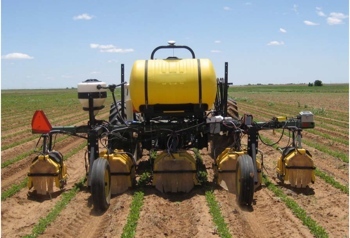
Figure 8. Typical deployment of WeedSeeker sprayers, under hoods in row crops, with three units under interior hoods and two units under exterior hoods.
