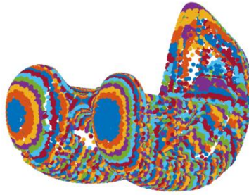
Figure 54. An example of a worse morphed CAD model needed to be smoothed: Multiple sections in one model.
